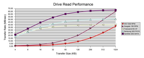
This is actually a very telling chart. It shows that Flash SSDs far outperform hard disks unless the transfer size is very large. Even a CF card outperforms a 15K SAS drive for block sizes of 256K or less.
