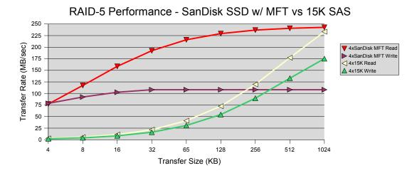
In order to equal the small block read and write performance of a 4 drive RAID-5 SanDisk SSD array with MFT, you would need a raid-10 array of about 80 15K SAS drives. The SSDs would draw about 3 watts of power while the SAS array would need nearly a kilowatt.
