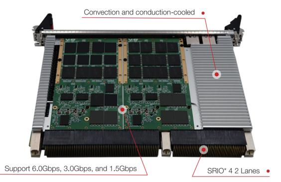
V&G 6U SRIO VPX is a high end data memory storage based on the FPGA customize design. It has 2 lane RapidIO \* 4 lines connector, single line can reach up to 6.25GB/s.
